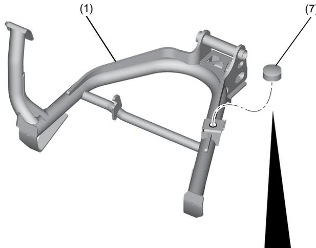
Apply synthetic detergent solution to  position shown.
